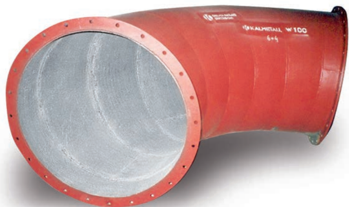
Pipe bends lined with KALMETALL in a de-dusting system application, the inner diameter is 400 mm, the system thickness is 8 + 5 mm.
