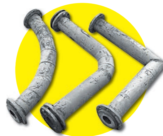
Pipe bend radius very strongly affects the extent of abrasion
