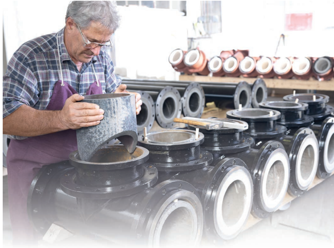
Assembly of the lining with cylinders
