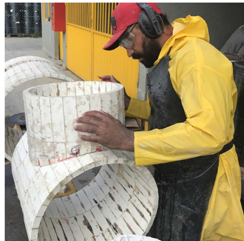
Pneumatic KALOCER transfer line with moulded components for conveying alternative fuel (demolition wood with sand particles) to a furnace, cross-section 203 mm
