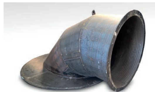
Pipe bends lined with KALMETALL in a de-dusting system application, the inner diameter is 400 mm, the system thickness is 8 + 5 mm.
