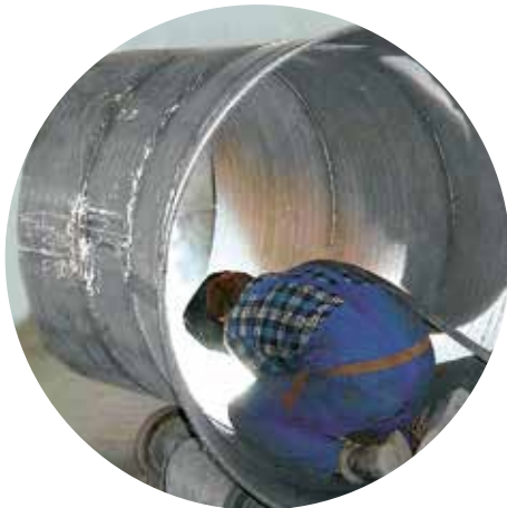
Large diameter dust collection pipes can be cost-effectively manufactured as selfsupporting structures of KALMETALL hard overlay welded plates.
