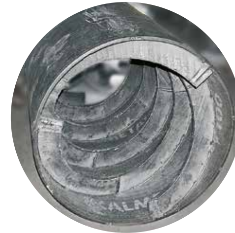
Both sides of the mill charger flights have been lined with KALMETALL W100; 800 mm diameter.
