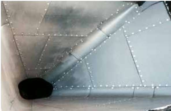
The slide promotion lining has raw materials continuously discharged from silos and bunkers without coating or clogging.
