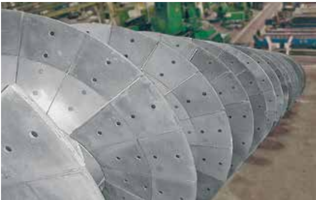
Screw conveyor protected with hard cast iron KALCAST. Depending on the alloy, a very high abrasion and impact resistance is achieved.
