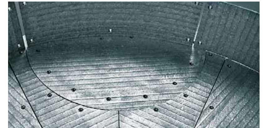
Both sides of the mill charger flights have been lined with KALMETALL W100; 800 mm diameter.
