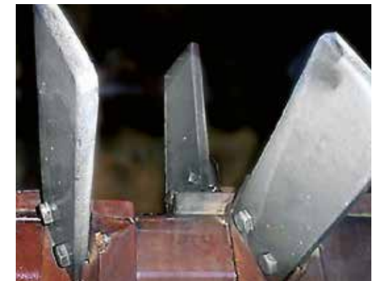
Paddles made of KALCAST 153 for a mineral washing system.
