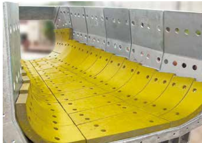
Reliable protection in a material chute with 62 mm thick KALCAST 155 castings. For improved impact resistance and noise level, an 8 mm thick rubber layer is installed beneath the castings.
