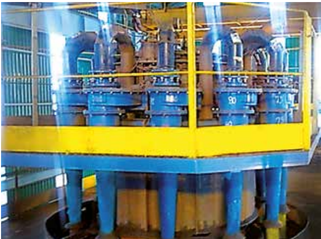
Proper wear protection of hydrocyclones extends the service life of the equipment and reduces the cost of downtime
