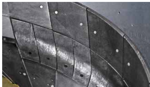
Reliable protection in a material chute with 62 mm thick KALCAST 155 castings. For improved impact resistance and noise level, an 8 mm thick rubber layer is installed beneath the castings.
