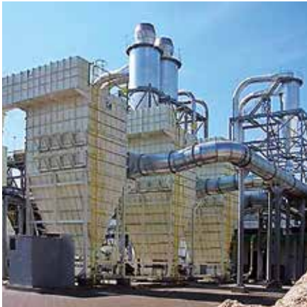
The fine dust that occurs in processing plants is extremely abrasive. This requires the plant components to be carefully protected. It is done both with metallic and ceramic materials.
