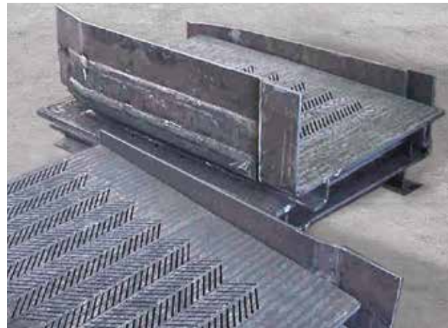
Reliable protection in a material chute with 62 mm thick KALCAST 155 castings. For improved impact resistance and noise level, an 8 mm thick rubber layer is installed beneath the castings.
