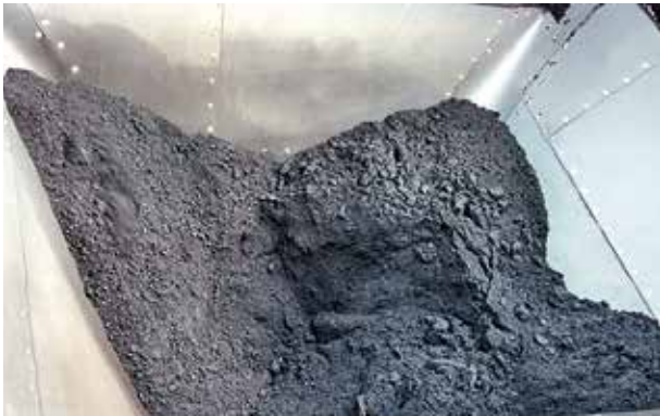
The slide promotion lining has raw materials continuously discharged from silos and bunkers without coating or clogging.
