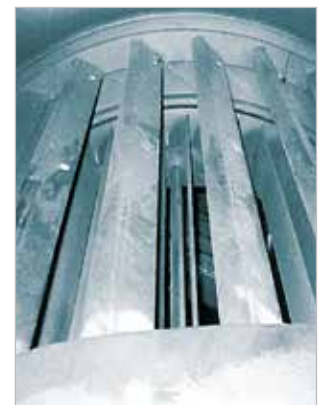
Weight saving design of a separator cage with KALSICA A silicon carbide ceramics; alternative linings are KALMETALL and KALOCER tiles.
