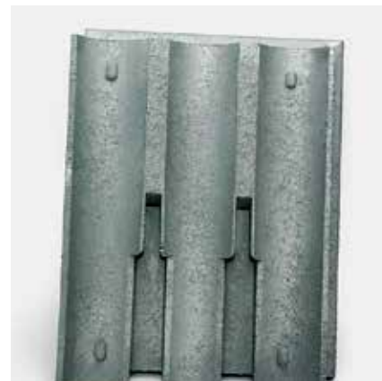
Solution adopted for economizers handling large dust quantities: tube protecting shapes made of KALSICA silicon carbide ceramics.
