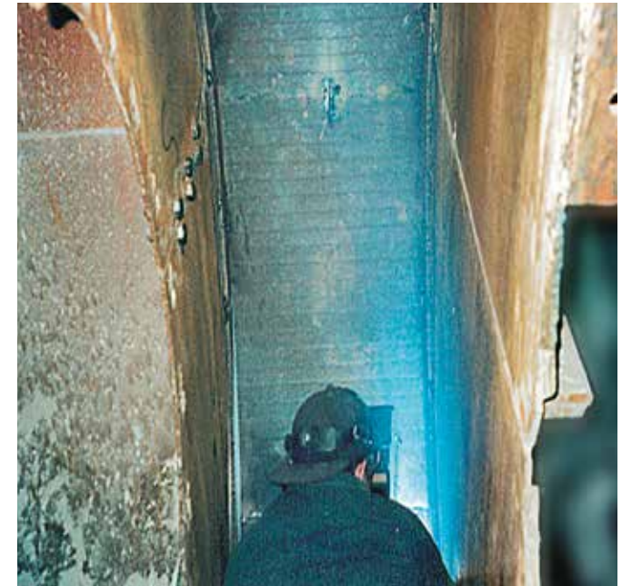
Housing of a pulverized coal fan protected with KALMETALL W100.
