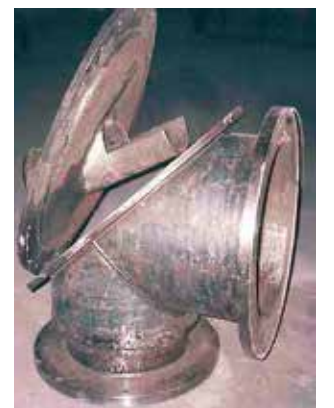
Pulverized coal burner made with parts of KALMETALL W100 hard overlay welding ready for installation.
