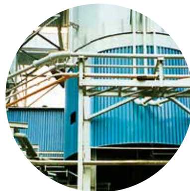
Limestone may have a very abrasive effect in FGD systems; a typical lining material is ABRESIST.
