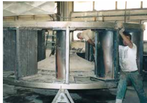
Impact coal pulverizers operate in lignite fired power plants; the impact plates are made of KALMETALL W100.
