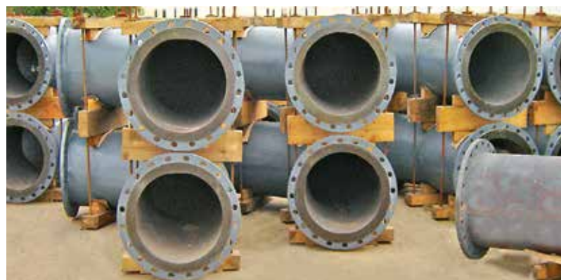
Long lifetimes at favorable costs are achieved with KALCAST hard casting; this example shows 518 mm diameter bends up to 700 kg weight.
