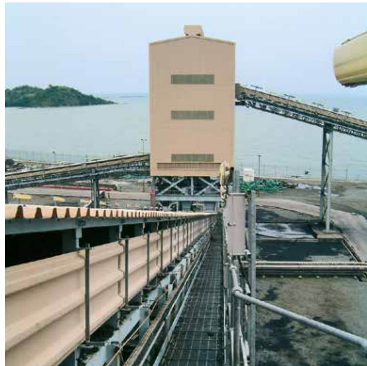
Coal transfer equipment is protected with ABRESIST fused cast basalt or KALOCER high alumina ceramics (example: Philippines).
