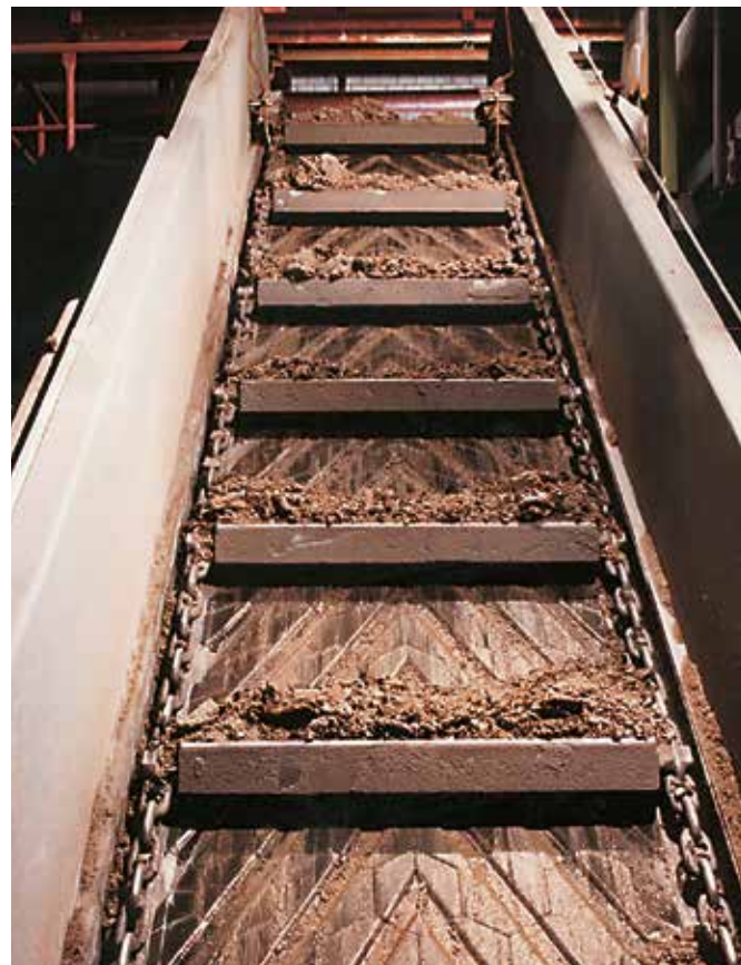
Chain conveyors for wet ash removal are efficiently lined with ABRESIST fused cast basalt; KALCOR, KALOCER or KALMETALL can be used as well.
