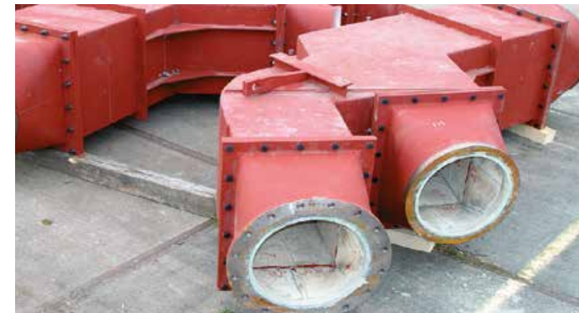
PF-distribution boxes protected with KALCOR for large area lining and KALOCER to ensure maximum wear resistance.
