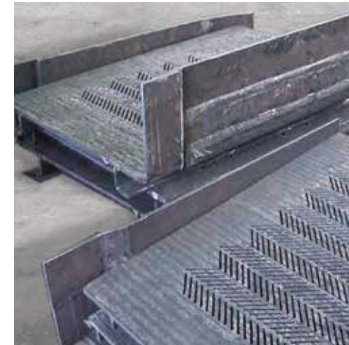
Screens for hot sintered material made of KALMETALL W145; the screen surface is of herringbone pattern
