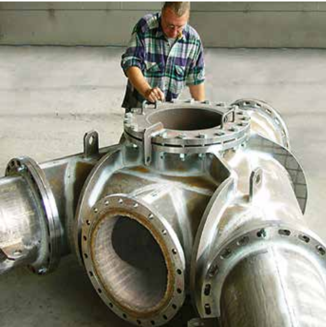
Pressure compensating pipe at the blast furnace; self-supporting structure of KALMETALL W100 30 + 6 hard overlay welding; 450 mm Ø
