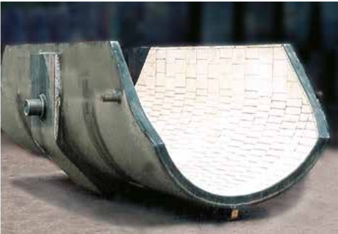
Distributor tilting chute being part of blast furnace lining fitted with KALOCER high-alumina ceramics, 50 mm thick
