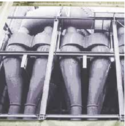
Depending on the specific plant design dust collection cyclones are protected either with ABRESIST fused cast basalt, KALCOR zirconium corundum, KALCRET hard compound or KALMETALL hard overlay welding
