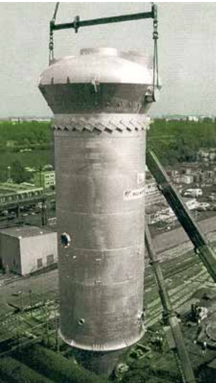
Dust collection cyclones for blast furnaces are effectively protected with combined linings
