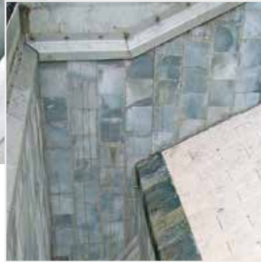
A trouble-free material flow is ensured in coal bunkers by the use of KALEN slide promotion plastics
