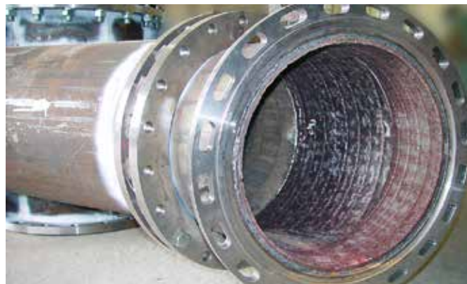
Pipe made of KALMETALL W100 hard overlay welding, inner diameter 500 mm
