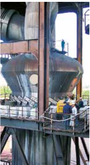
Short lining times for a whirler are achieved with a combined lining of hard compound KALCRET BTS and zirconium corundum KALCOR. The high application rate of KALCRET BTS is 5 m 2 /h
