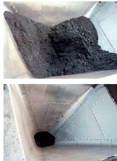
Bunker for fine coal: The slide promoting lining ensures the material flow without sticking and clogging.
