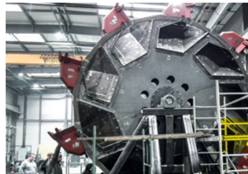
A bucket wheel as an example of tailor-made KALMETALL welded construction
