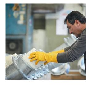
Green pipes and pipe bends have a wear-resistant lining that can be removed and recycled at the end of their service life.
