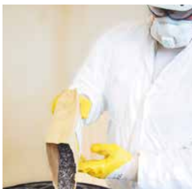
Add fibre components slowly and continuously and mix dry for about 1 minute
