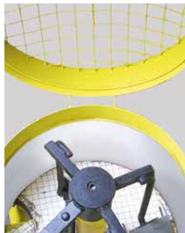
Wear protected tank of the Kalenborn forced circulation mixer
