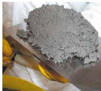
The stiff / plastic KALCRET compound (X) to be applied by trowelling with the aid of simple bricklayer tools
