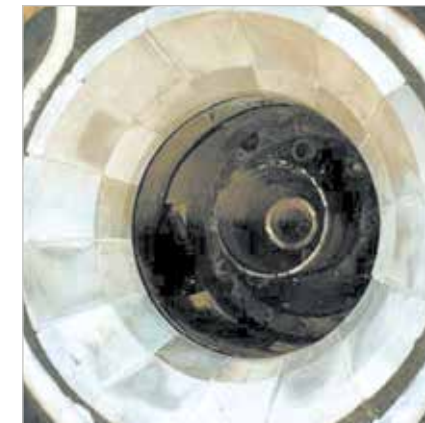
Burner cone for a power station made of KALSICA
