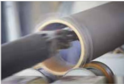
Wear-resistant pipe with KALEA high-performance plastic
