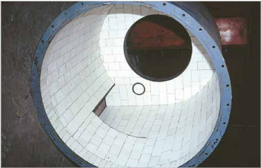
Lining of a cyclone handling diatomaceous earth lined with 6 mm thick KALOCER tiles; the epoxy setting is resistant up to 180 °C / 356 °F
