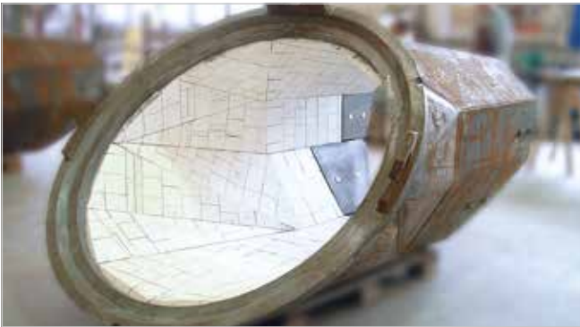
Octagonal hopper in a steel plant; the 50 mm thick KALOCER tiles have been three-dimensionally shaped and cut
