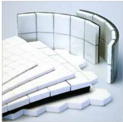
Kalenborn offer KALOCER mosaics in different sizes: square, hexagonal or special design from 1,5 mm to 12 mm thickness. Mosaics can be supplied with book ends. Vulcanized solutions are available.
