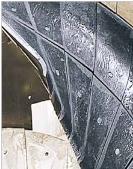
Shaft flight of KALCAST proven in use for hard coal mining
