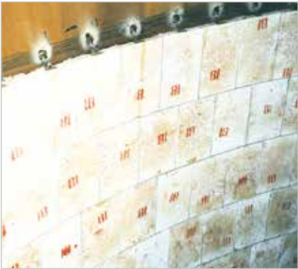
High temperature wear protection in a dedusting cyclone of a blast furnace plant in Europe
