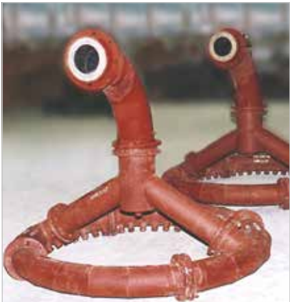
Separator components provided with ABRESIST wear protection
