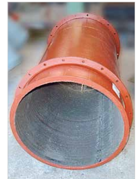
Pipe armored with KALMETALL installed in a dust collecting system; inside diameter 400 mm, system thickness 8 + 5 mm
