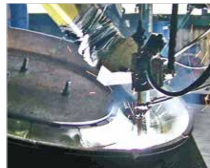
Kalenborn welding service, regeneration of a grinding table
