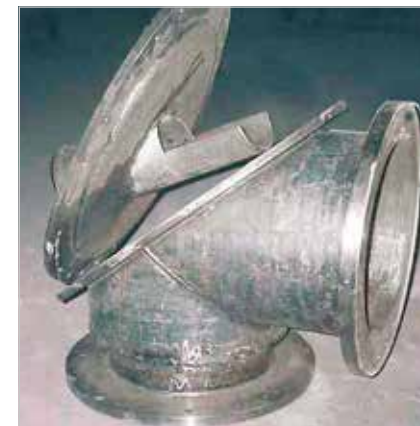
Pulverized coal burner lined with KALMETALL
