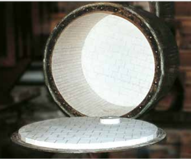
KALOCER lining of a mill for superfine grinding of coloured pigments
