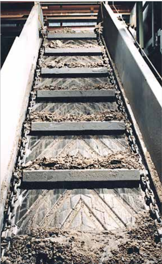
Chain conveyor for wet ash removal in a power plant. Drains cast into the lining reduce the undesired carrying of water to the discharge zone thereby lowering the water consumption rate.
