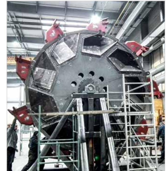
For a steel manufacturer in North Africa, a bucket wheel as a custom KALMETALL welded construction
