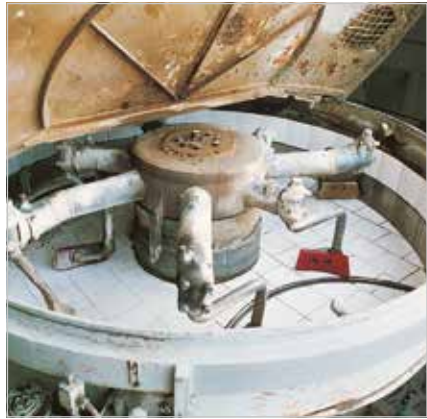
Agitators and mixers subject to extreme wear can be durably protected with KALOCER tiles shaped to the specific equipment design
