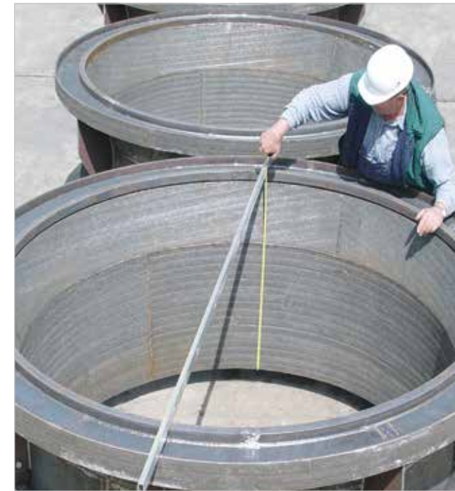
Separating cones of cement classifiers made of KALMETALL as self-supporting structures
