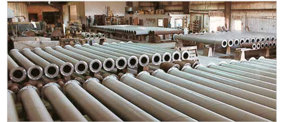
Hydraulic ash conveying pipe being manufactured at the Abresist Kalenborn Corporation plant in Indiana, USA
