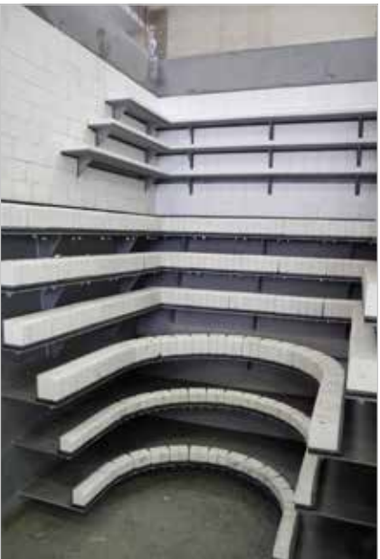
Cascade chute with wear blocks made of 100-mm-thick KALOCER oxide ceramic. The ceramic is fixed to the impact plates in KALFIX setting compound. The impact plates are fastened to the chute with an angle bracket.
