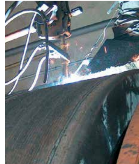
Service by Kalenborn: rebuilding of a grinding roll with KALMETALL W100
