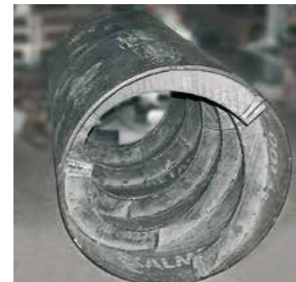
Both sides of the mill charger flights have been lined with KALMETALL W100; 800 mm diameter.
