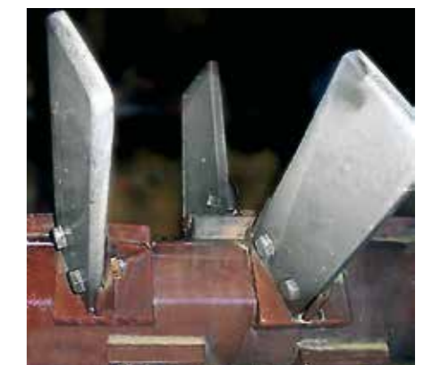
Paddles made of KALCAST 153 for a mineral washing system.
