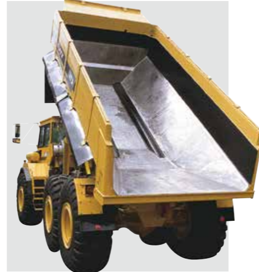
Dump trucks require special lining. KALMETALL is especially useful. KALINOX and KALEN are given preference for handling sticky materials.
