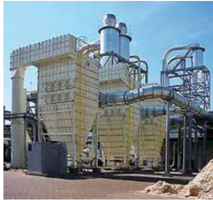
The fine dust that occurs in processing plants is extremely abrasive. This requires the plant components to be carefully protected. It is done both with metallic and ceramic materials.
