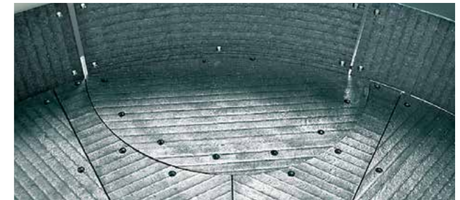
Lining of a mixer: the sidewalls, the bottom and the discharge elements have been protected with KALMETALL W100; diameter 3.500 mm.
