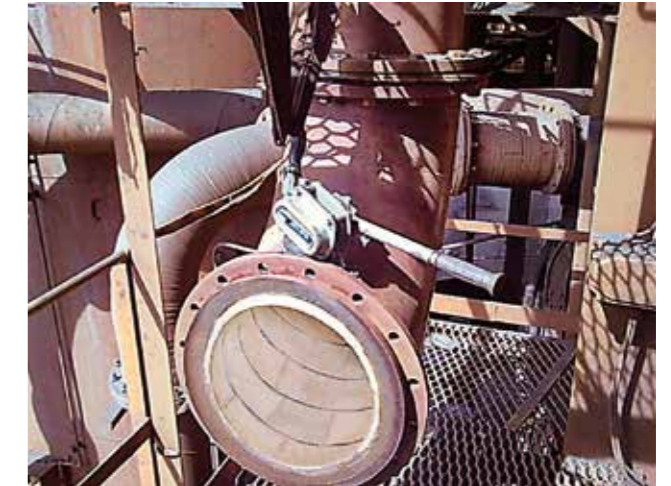
Pipes protected with KALCOR zirconium corundum installed in the discharge section of an iron ore grinding mill in Brazil. Rubber linings failed after a few months whereas the KALCOR lining has been in operation for several years.
