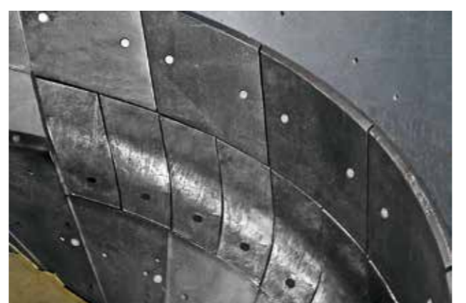
Screens are used in many areas of raw material processing. The herringbone pattern is burned in the KALMETALL hard overlay welded plates.
