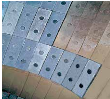
Lining of an infeed coal pulverizer with KALCAST.
