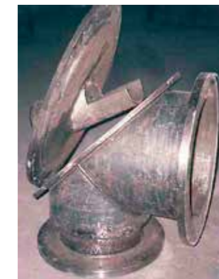
Pulverized coal burner made with parts of KALMETALL W100 hard overlay welding ready for installation.
