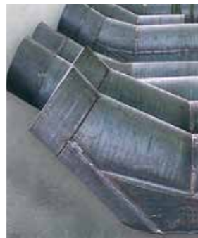
Reliable wear protection is of particular importance for trouble-free continuous operation of the pulverised coal burners.
