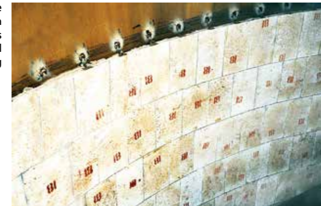
Short lining times for a whirler are achieved with a combined lining of hard compound KALCRET BTS and zirconium corundum KALCOR. The high application rate of KALCRET BTS is 5 m 2 /h
