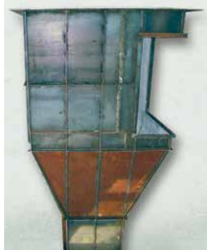
KALCRET hard compound has stood the test as lining material in components of slag granulating systems. Depending on their specific geometry the plant components can be lined within a minimum of time by trowelling or by the spraying technique.
