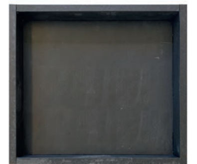
Plastic sample form: 320 x 300 x 40 mm
