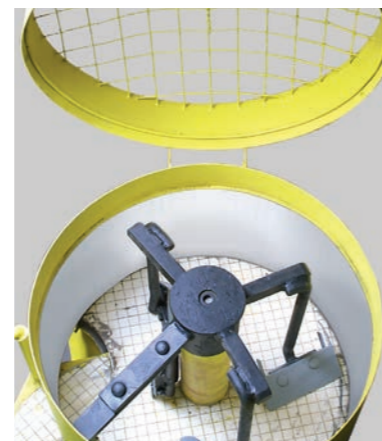
Wear protected tank of the Kalenborn forced circulation mixer
