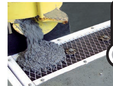
2. Prepare cast compound as instructed
