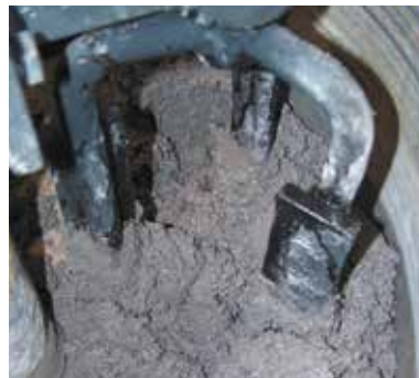
The compound should have a stiff / plastic consistency
