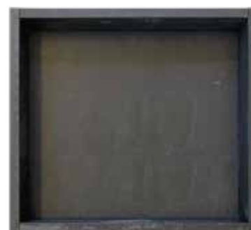
Plastic sample form: 320 x 300 x 40 mm
