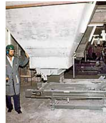
Limestone bunker with slide promoting lining made of KALEN 1006
