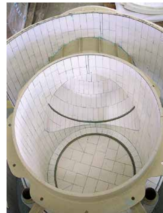
Precise fitting of KALOCER high alumina ceramics, 13 and 25 mm thick
