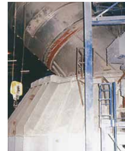
Protection of a raw meal mill: KALCRET for the duct, KALMETALL W100 for the mill lining
