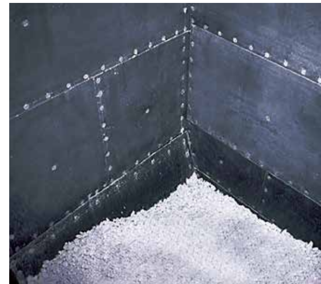
Protection of a raw meal mill: KALCRET for the duct, KALMETALL W100 for the mill lining
