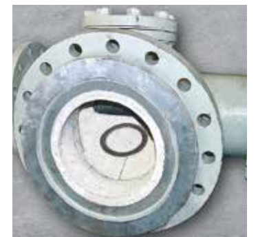
Pipe diverter in pneumatic pipe lined with KALCOR
