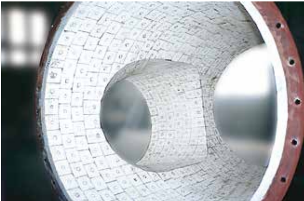
KALOCER high alumina ceramics lining of a separator with mechanically fixed tiles, approx. 100 x 100 mm
