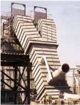
Cooler waste gas pipe lined with KALCRET BNY hard compound
